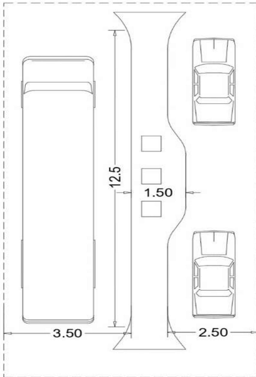
Figure 13: Schematic layout for the charging station
