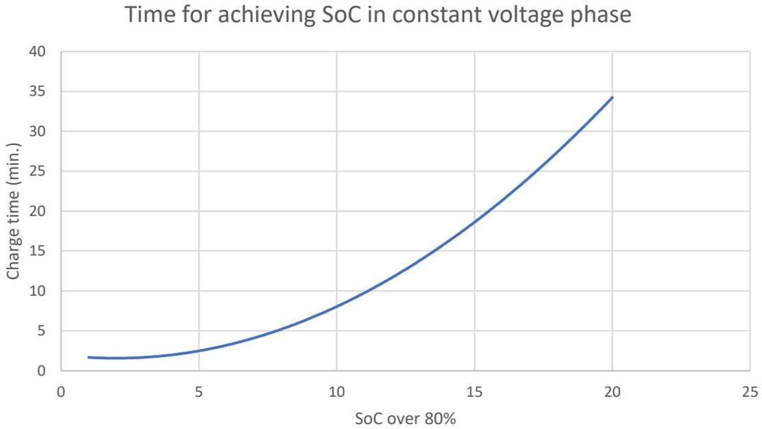
Figure 4: Time to achieve SoC level over 80% SoC in constant voltage phase
