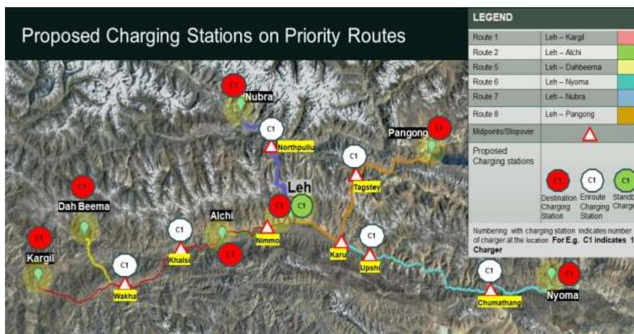
Figure 12: Routes with proposed charging stations
