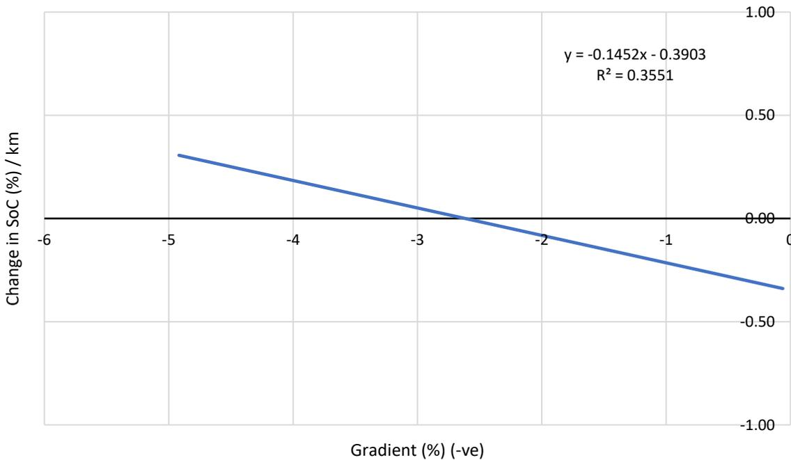
Figure 5: Relationship between gradient and percentage change of SoC from that on flat terrain
