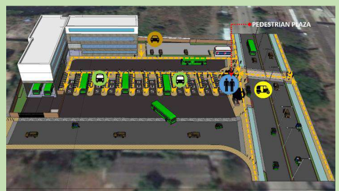
Figure 33: Pedestrian circulation in bus terminal
